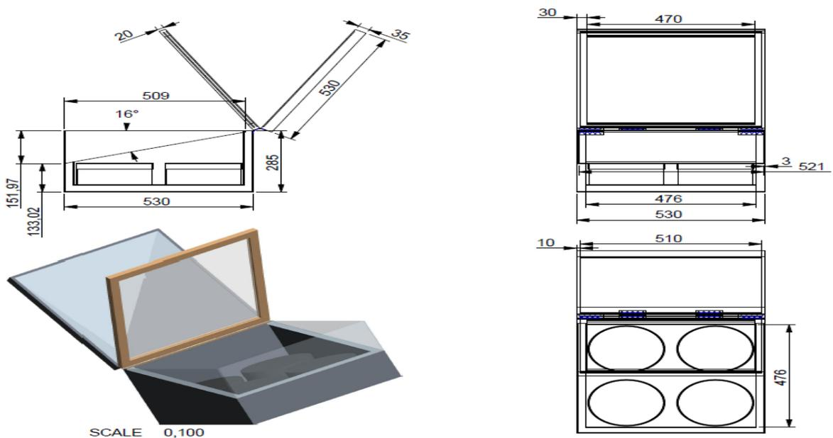
Figure II: Solar Cooker of  $\beta=16^\circ$
