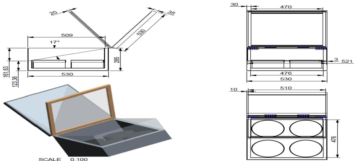
**Figure III: Solar Cooker of  $\beta=17^\circ$**
