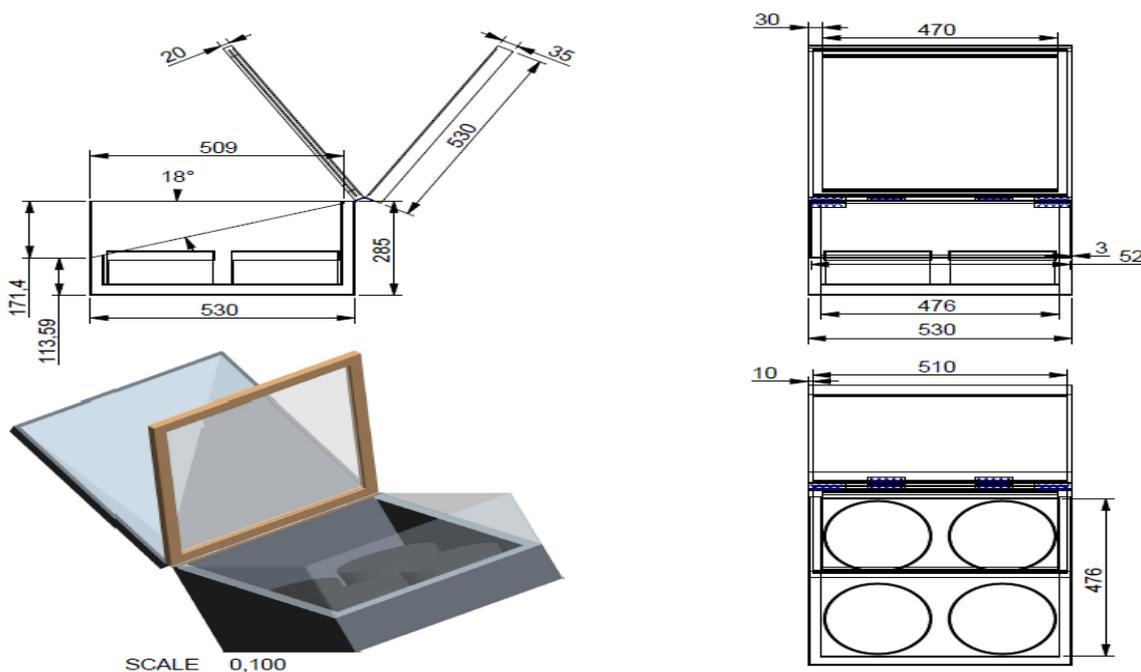
**Figure IV: Solar Cooker of  $\beta=18^\circ$**
