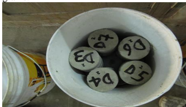
Fig 2: Setup of hot water curing
