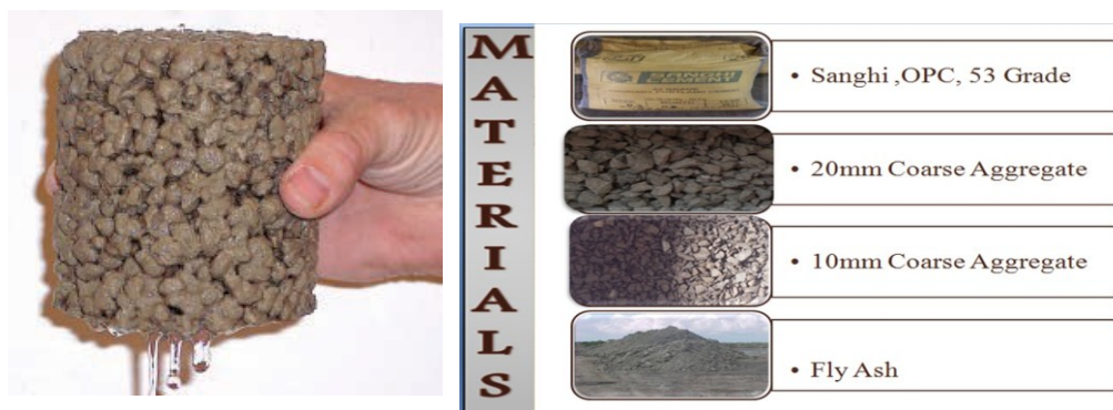
Figure 1: Pervious concrete materials
