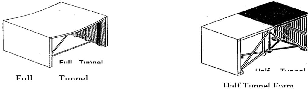
(a) U or Inverted L shape Steel Tunnel Forms
