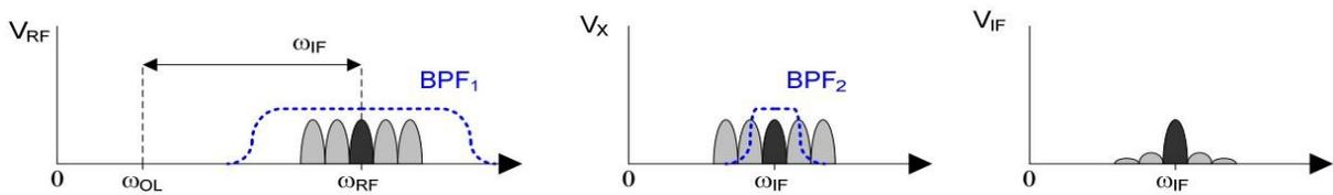
Figure 2: Band Selecting and Channel Filtering [3].
