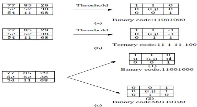
Fig. 3. (a) The LBP operator, (b) LTP operator, and (c) TheTan and Triggs LTP operator.
