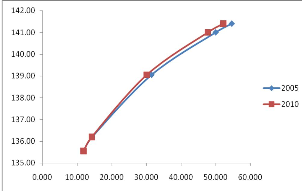
Fig 2. Capacity- Elevation curves for year 2005 and 2009/10
