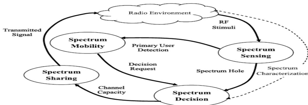
Figure 2.5 The cognitive radio cycle
