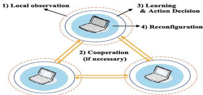
Figure 2.4 Cognitive Radio Ad-Hoc Network
