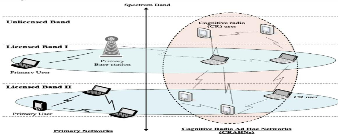
Figure 2.3 - The CRAHN architecture
