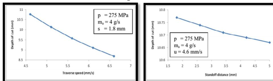
**Figure 5 (c) Traverse speed versus depth of cut, (d) Standoff distance versus depth of cut**
