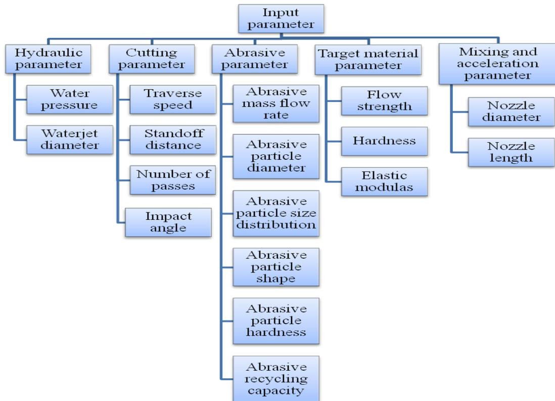
**Figure 2 Input parameters of AWJM**
