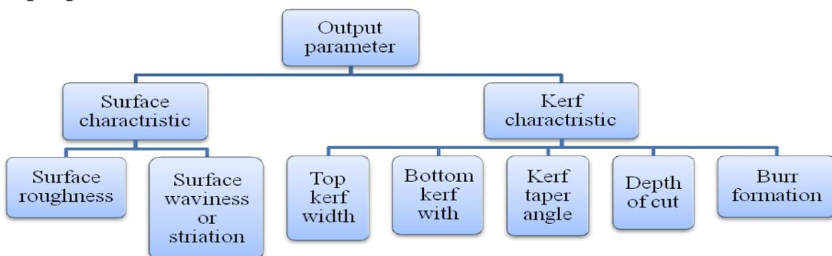
**Figure 3 Output parameters of AWJM**
