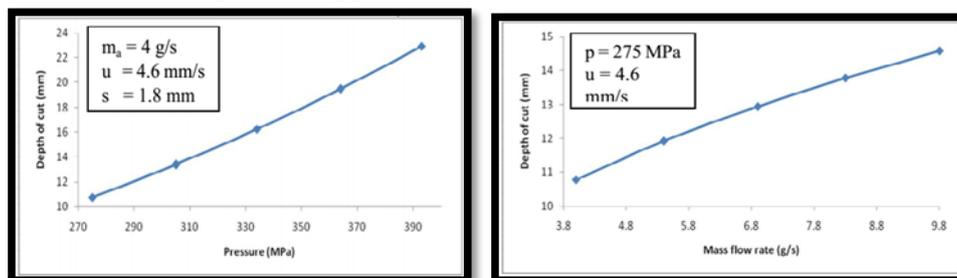
**Figure 4 (a) Water pressure versus depth of cut, (b) Abrasive mass flow rate versus depth of cut**
