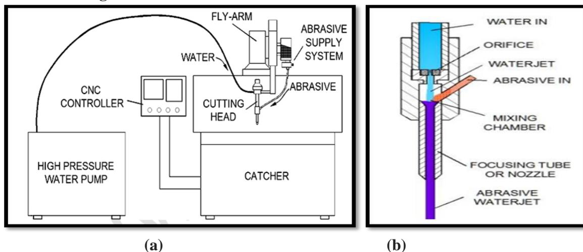
**Figure 1 (a) Schematic diagram of AWJM, (b) Inside AWJ generator**
