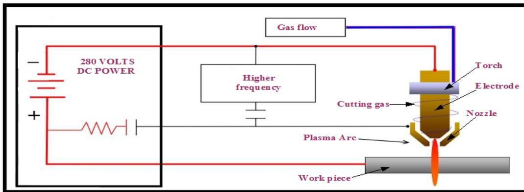
**Figure 1.2: Plasma Arc Cutting Schematic Diagram**
