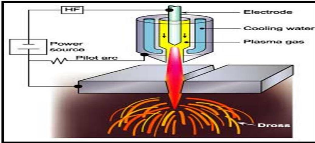
**Figure 1.1: Plasma Arc Cutting** [2]
