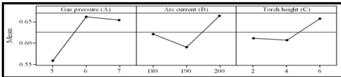
Figure 2.1: Main effects is plot for mean of grey relational grade<sup>[1]</sup>
