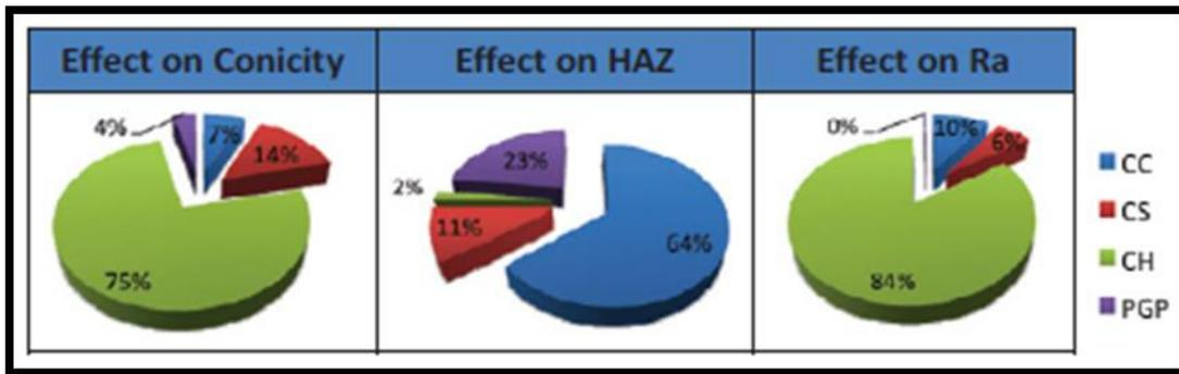
**Figure 2.2: Effect of process parameters on Conicity, HAZ and Ra**<sup>[2]</sup>
