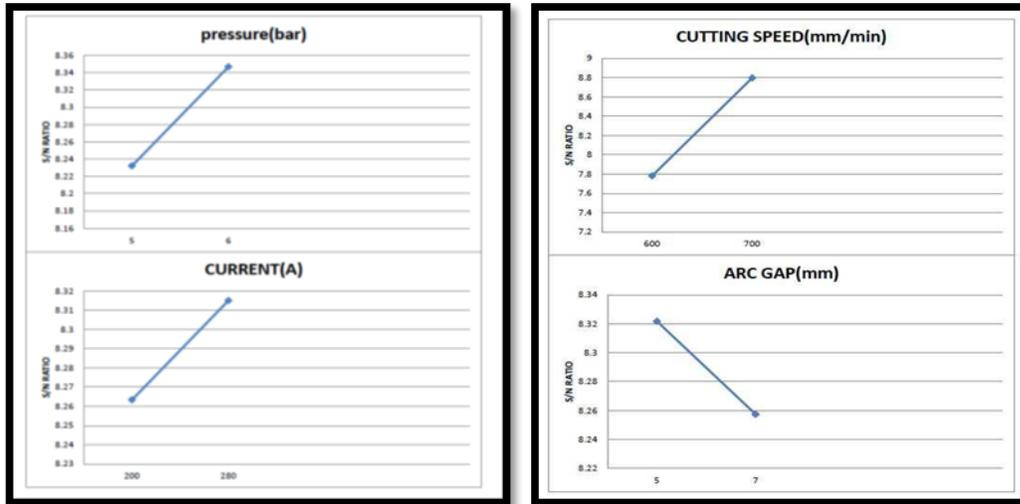
**Figure 2.3: Effect of Pressure & current On MRR** **Figure 2.4: Effect of Cutting speed & ARC GAP on MRR**
