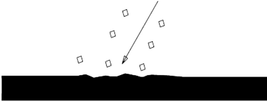
**Fig: 1.3 Erosive Wear**
