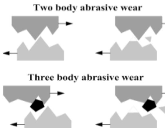
**Fig 1.1 Abrasive Wear**
