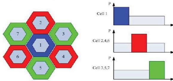
Fig 8. The frequency planning and power allocation for the SFR scheme [3]
