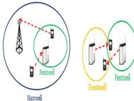
Fig 1. Cross tier interference Fig 2. Co-tier interference [4]
