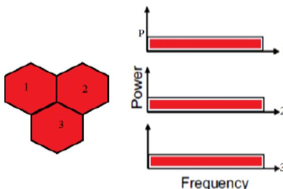
Fig 5. Frequency and power allocation (Reuse-1) <sup>[2]</sup>
