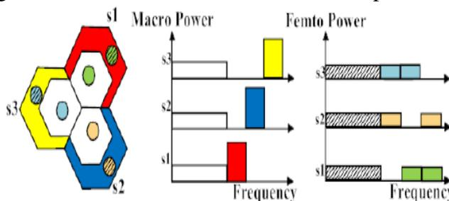
Fig 9. Partial Frequency Reuse [2]
