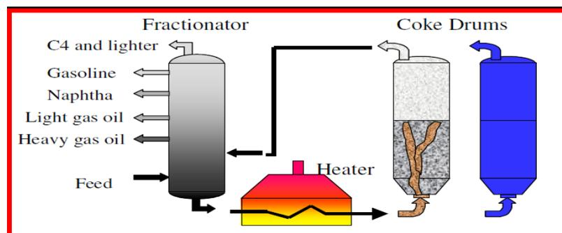
Figure-1 Simple Flow Diagram of delayed coking unit <sup>[3]</sup>
