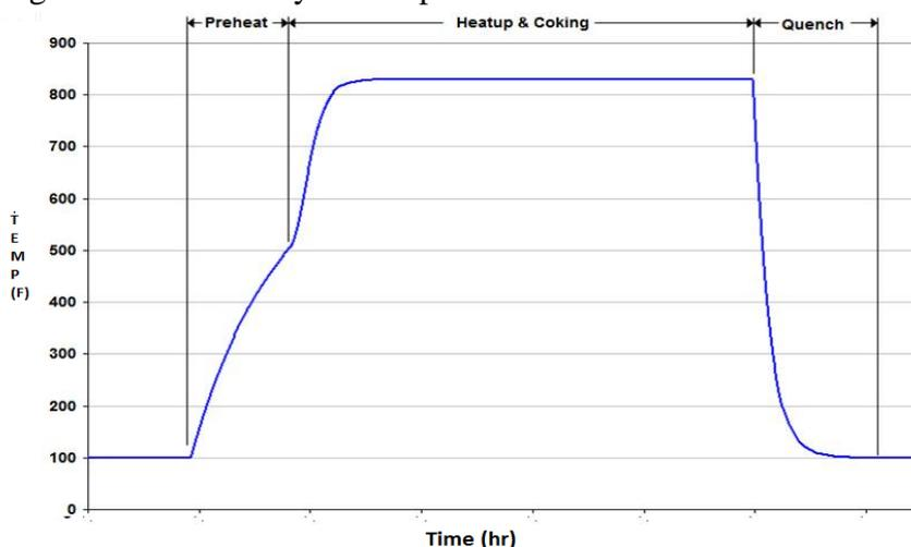
Figure-2 Coke drums operation cycle <sup>[5]</sup>
