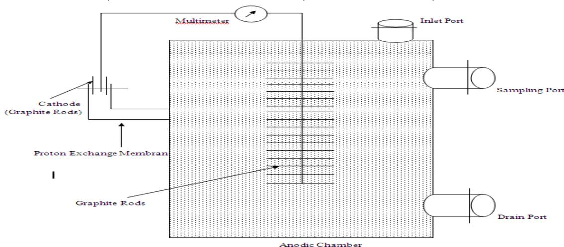
**Figure1: Single Chambered Microbial Fuel Cell**
