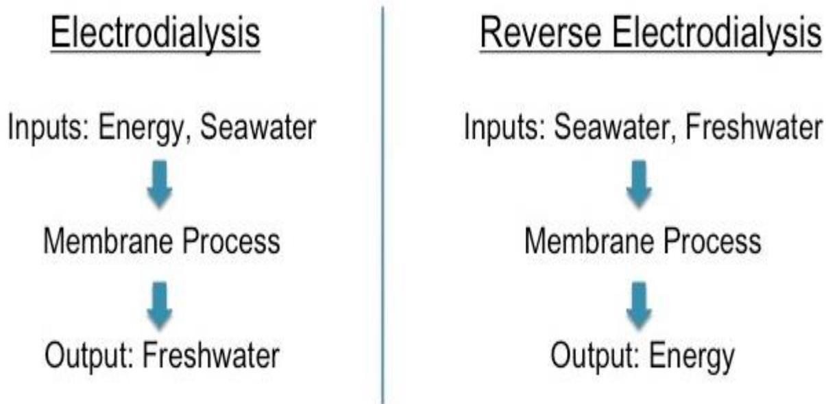
**Figure 1:** Conceptual flow for ED and RED membrane processes
