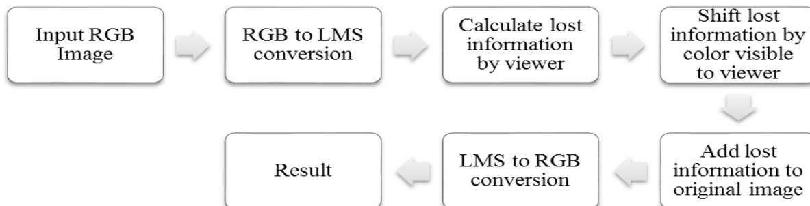
Figure 2: Block diagram of LMS daltonization
