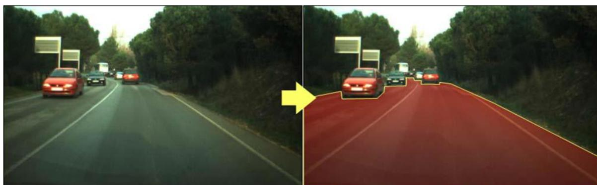
**Figure 1: Goal of vision-based road detection is identifying road pixels in an image <sup>[10]</sup>**
