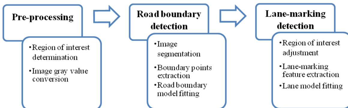
Figure 3: Basic block diagram of road detection <sup>[1]</sup>
